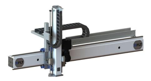
THE LGR-5 IS DESIGNED FOR HANDLING WEIGHTS OF UP TO 1400 KG, MASTERS VERTICAL STROKES UP TO APPROX. 3.5 M AND REACHES A MOVEMENT SPEED OF UP TO 4.5 M/S WITH ACCELERATION OF UP TO 6 M/S<sup>2</sup>.
