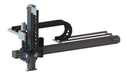
THE LGR-2 IS DESIGNED FOR HANDLING WEIGHTS OF UP TO 150 KG, MASTERS VERTICAL STROKES UP TO APPROX. 2.5 M AND REACHES A MOVEMENT SPEED OF UP TO 4.5 M/S WITH ACCELERATION OF UP TO 6 M/S<sup>2</sup>.
