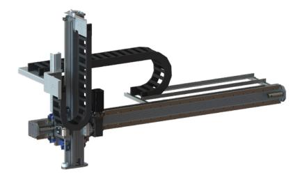
THE LGR-1 IS DESIGNED FOR HANDLING WEIGHTS OF UP TO 80 KG, MASTERS VERTICAL STROKES UP TO APPROX. 3 M AND REACHES A MOVEMENT SPEED OF UP TO 4.5 M/S WITH ACCELERATION OF UP TO 6 M/S<sup>2</sup>.
