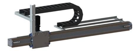
THE LHA-2 IS DESIGNED FOR HANDLING WEIGHTS OF UP TO 275 KG AND REACHES A MOVEMENT SPEED OF UP TO 4.5 M/S WITH ACCELERATION OF UP TO 6 M/S<sup>2</sup>.
