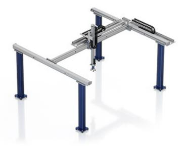
THE AGR-6 IS DESIGNED FOR HANDLING WEIGHTS OF UP TO 1400 KG, MASTERS VERTICAL STROKES UP TO APPROX. 3.5 M AND REACHES A MOVEMENT SPEED OF UP TO 1 M/S WITH ACCELERATION OF UP TO 2 M/S2.
