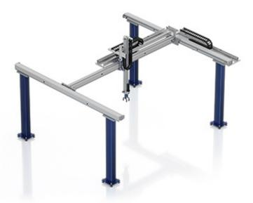
THE AGR-3 IS DESIGNED FOR HANDLING WEIGHTS OF UP TO 250 KG, MASTERS VERTICAL STROKES UP TO APPROX. 3 M AND REACHES A MOVEMENT SPEED OF UP TO 2 M/S WITH ACCELERATION OF UP TO 4 M/S<sup>2</sup>.
