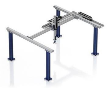
THE AGR-2 IS DESIGNED FOR HANDLING WEIGHTS OF UP TO 150 KG, MASTERS VERTICAL STROKES UP TO APPROX. 2.5 M AND REACHES A MOVEMENT SPEED OF UP TO 2 M/S WITH ACCELERATION OF UP TO 4 M/S<sup>2</sup>.
