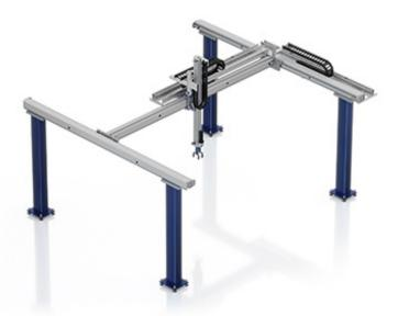
THE AGR-1 IS DESIGNED FOR HANDLING WEIGHTS OF UP TO 80 KG, MASTERS VERTICAL STROKES UP TO APPROX. 2 M AND REACHES A MOVEMENT SPEED OF UP TO 2 M/S WITH ACCELERATION OF UP TO 4 M/S<sup>2</sup>.
