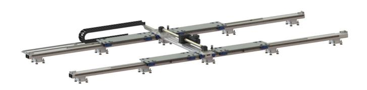
THE LFA-5 IS DESIGNED FOR HANDLING WEIGHTS OF UP TO 5000 KG AND REACHES A MOVEMENT SPEED OF UP TO 3 M/S WITH ACCELERATION OF UP TO 3 M/S<sup>2</sup>.
