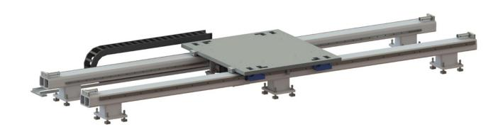
THE LFA-4 IS DESIGNED FOR HANDLING WEIGHTS OF UP TO 2000 KG AND REACHES A MOVEMENT SPEED OF UP TO 4 M/S WITH ACCELERATION OF UP TO 4 M/S<sup>2</sup>.
