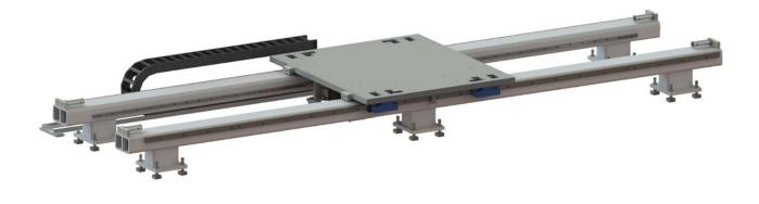
THE LFA-2 IS DESIGNED FOR HANDLING WEIGHTS OF UP TO 600 KG AND REACHES A MOVEMENT SPEED OF UP TO 4.5 M/S WITH ACCELERATION OF UP TO 6 M/S<sup>2</sup>.
