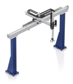
THE AGC-6 IS DESIGNED FOR HANDLING WEIGHTS OF UP TO 600 KG, MASTERS VERTICAL STROKES UP TO APPROX. 3 M AND REACHES A MOVEMENT SPEED OF UP TO 1 M/S WITH ACCELERATION OF UP TO 2 M/S<sup>2</sup>.
