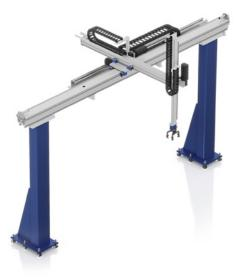
THE AGC-4 IS DESIGNED FOR HANDLING WEIGHTS OF UP TO 450 KG, MASTERS VERTICAL STROKES UP TO APPROX. 3 M AND REACHES A MOVEMENT SPEED OF UP TO 1 M/S WITH ACCELERATION OF UP TO 2 M/S<sup>2</sup>.
