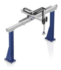
THE AGC-4 IS DESIGNED FOR HANDLING WEIGHTS OF UP TO 350 KG, MASTERS VERTICAL STROKES UP TO APPROX. 3 M AND REACHES A MOVEMENT SPEED OF UP TO 2 M/S WITH ACCELERATION OF UP TO 4 M/S<sup>2</sup>.
