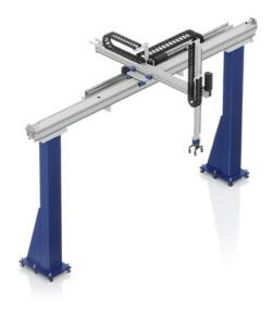
THE AGC-2 IS DESIGNED FOR HANDLING WEIGHTS OF UP TO 90 KG, MASTERS VERTICAL STROKES UP TO APPROX. 2.5 M AND REACHES A MOVEMENT SPEED OF UP TO 2 M/S WITH ACCELERATION OF UP TO 4 M/S<sup>2</sup>.
