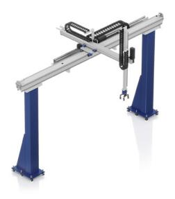
THE AGC-1 IS DESIGNED FOR HANDLING WEIGHTS OF UP TO 25 KG, MASTERS VERTICAL STROKES UP TO APPROX. 2 M AND REACHES A MOVEMENT SPEED OF UP TO 2 M/S WITH ACCELERATION OF UP TO 4 M/S<sup>2</sup>.
